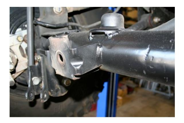
3. Attach the new track bar relocation bracket to the factory bracket as shown with the new 9/16" bolt and lock nut; use a flat washer under the bolt head and lock nut.
