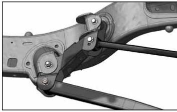
**Note:** It may be easier to align the control arms to the mount by removing the opposite side upper control arm and adjusting the axle with a hydraulic jack.
