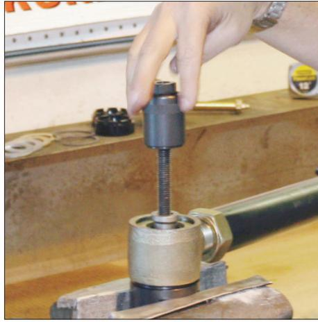
5) With the snap ring removed, you may now back the press nut off to release the load on the internals of the Johnny Joint®. Once the load is relieved, you may spin the press nut back off of the threads of the tool and remove the nut and the tool from the tool base.
