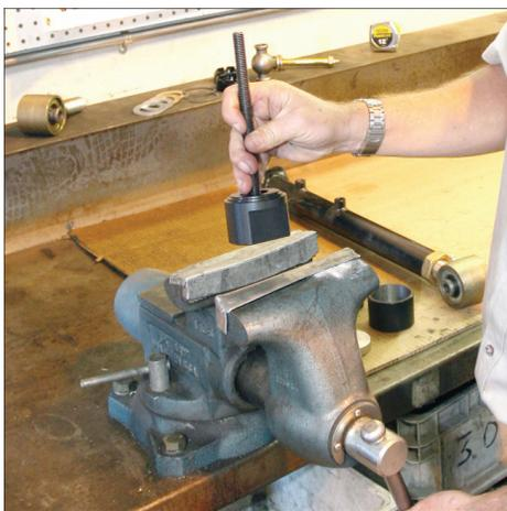
**1)** Start by installing the base of the tool in a sturdy bench vise.
