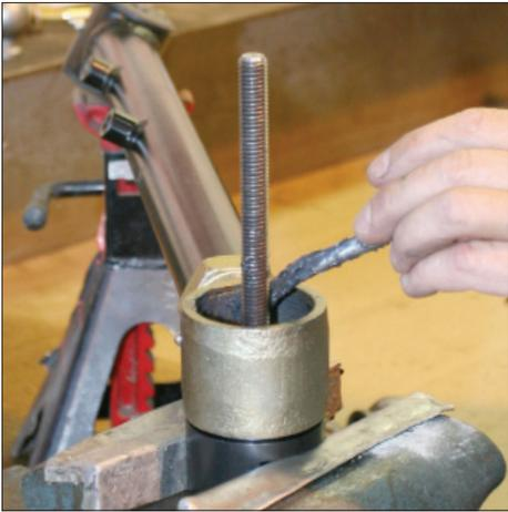
1) Thoroughly clean the Johnny Joint® outer shell, then index it onto it's shoulder on the tool base - make sure the snap ring groove side is up. Before installing the internals, grease the inside of the shell with good quality, non-synthetic moly lube - we use Chevron brand name.
