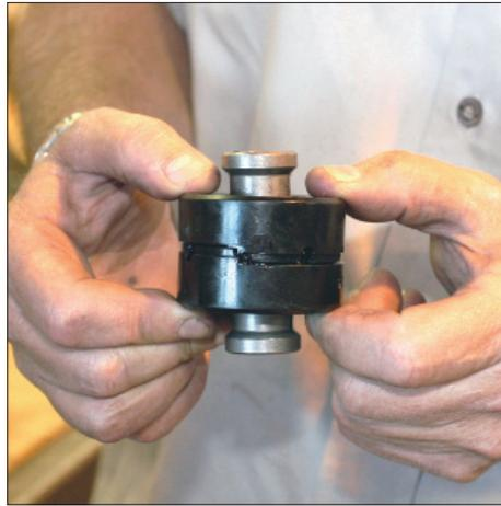
2) Grease the ball center with the moly lube, and then preassemble it with the bushings. The bushings interlock and are not a male/female style. Make sure the bushings are fully interlocked before attempting further assembly.
