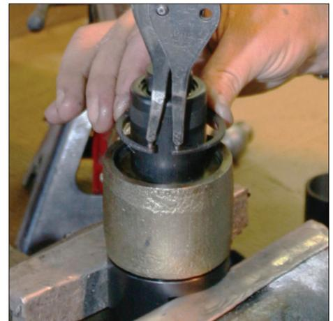
6) With the press nut still in place, remove the sleeve, and give the snap ring groove another close look for debris. During the installation of the internals, urethane can be scraped off of the bushings and into the groove. After you have ensured the groove is clean, you may install your snap ring. Make sure the snap ring is installed sharp side of it's stamping out.
