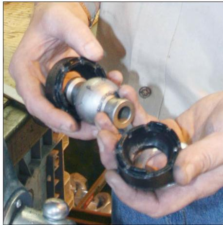
8) You may now disassemble, clean, and inspect the Johnny Joint® internals. Wear on the ball center can generally be cleaned with emory cloth and the ball center reused. Bushings that are worn, washers that are bent, and snap rings that are bent or showing wear should be replaced. Thoroughly clean the outer shell. Carefully inspect the snap ring groove for debris, and then remove any dirt, grease, or urethane that is found.
