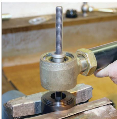
**2)** Slide the Johnny Joint® that you will be disassembling onto the threads of the tool, making sure the snap ring side is facing up! The outer shell of the Johnny Joint® will lock into one of the machined shoulders on the tool's base.
