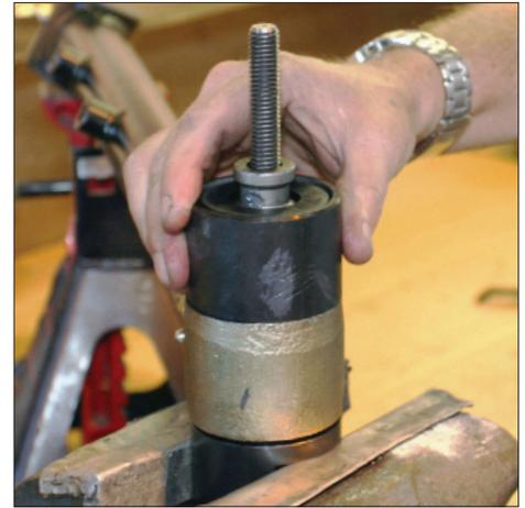
3) Put the sleeve on top of the Johnny Joint® small side down, install the lower washer first, and then install the internals. NOTE: examine the washer to make sure you are installing it with the sharp side of the washer stamping out.
