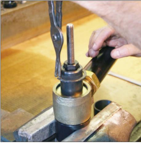
4) Remove the snap ring with a pair of good quality snap ring pliers. Straight or angled style will work.
