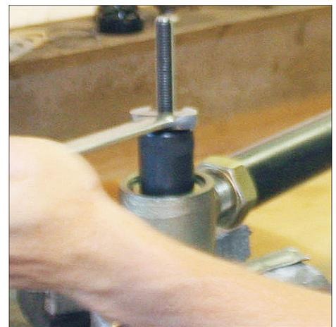
**3)** Spin the press nut on by hand until it reaches the side washer of the Johnny Joint®. Then with the proper wrench, tighten the press nut to compress the urethane inside the joint. You only need to tighten the press nut enough to release the load off of the snap ring.
