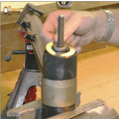
4) Install the outside washer. Again, ensure that it is being installed with the sharp side of the stamping of the washer away from the urethane.
