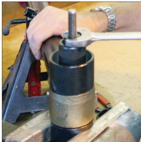
5) Run the press nut back on by hand until it's snug. Tighten it only enough to allow the snap ring to be installed. Over-tightening can cause the new side washers to bend.
