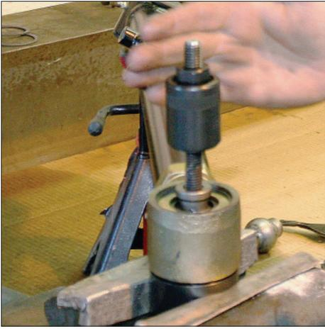
7) Release the tension on the press nut and then spin it off of the threads of the tool. The Johnny Joint® is now complete. Give it one more final inspection, and don't forget to grease it before use! Regular greasing will provide long Johnny Joint® life.
